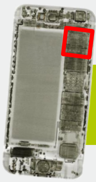
1a 3D CT Scan of a smartphone with chip package highlighted in red
